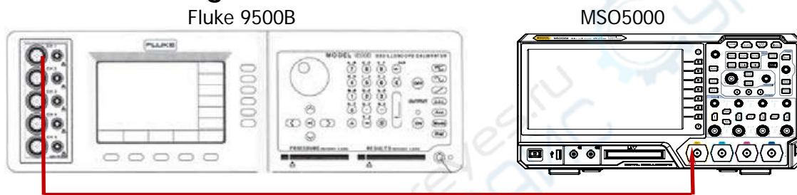
Figure 2-4 Bandwidth Limit Test Connection Diagram
