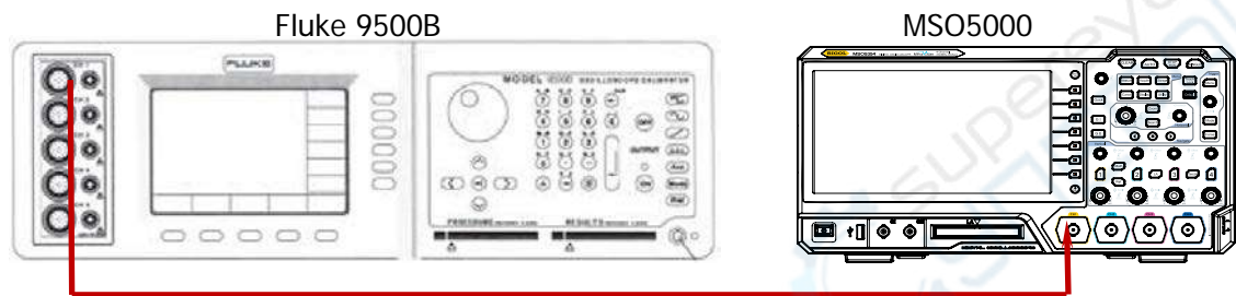
Figure 2-2 DC Gain Accuracy Test Connection Diagram
