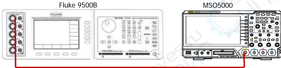
Figure 2-3 Bandwidth Test Connection Diagram
