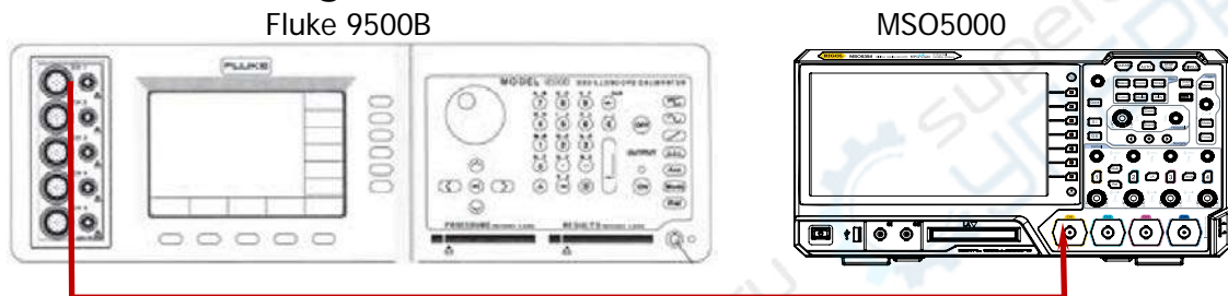
Figure 2-5 Timebase Accuracy Test Connection Diagram
