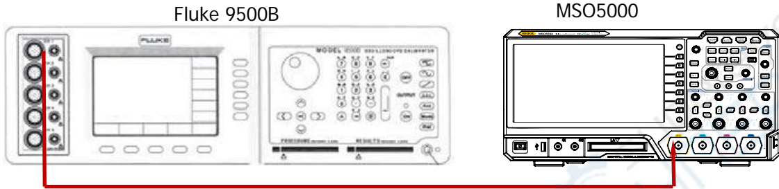
Figure 2-1 Impedance Test Connection Diagram
