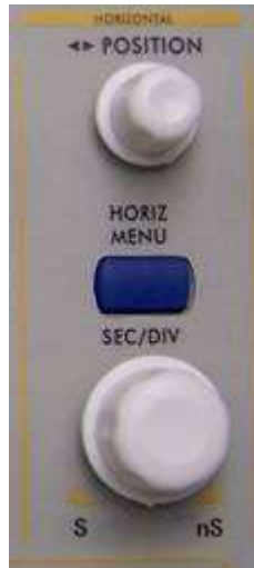
Fig. 4-10 Horizontal Control Zone
